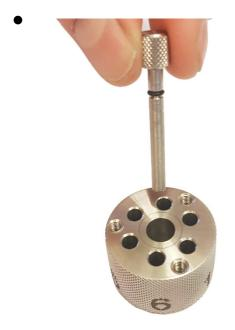
Remove the cartridges or empty shell casings from the drum. If necessary, use the ejector to eject the shell cases from the front of the drum.
