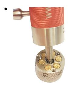
Hold the filled drum with one hand and guide the axis of the main unit through the drum with the other hand.
