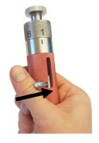
Use your thumb to push the cocking lever to the right until it jumps out of the locking position and fires the cartridge.
